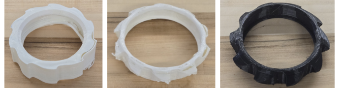
Fig. 14. Before and after adjusting print parameters and design to improve manufacturing quality. The main changes were that supports were enabled during printing, and flat surfaces were minimized in the design.
