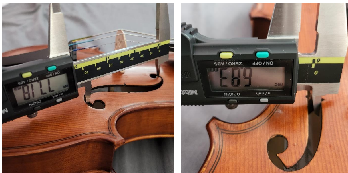
FIGURE 2.4. F-hole overall dimensions on the cheap violin.
