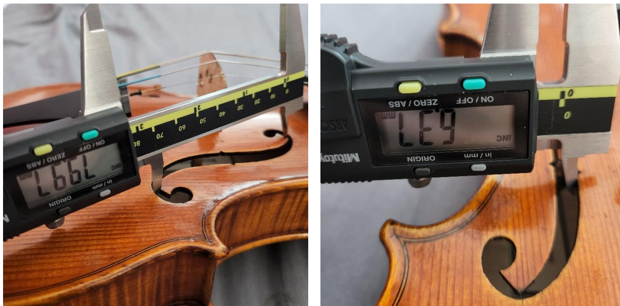
FIGURE 2.3. F-hole overall dimensions on the expensive violin.
