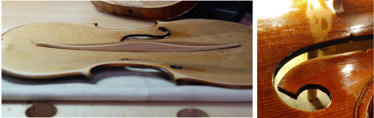
FIGURE 1.11. Bass bar being fitted on a violin (left), sound post viewed through the f-hole (right) [21,22].
