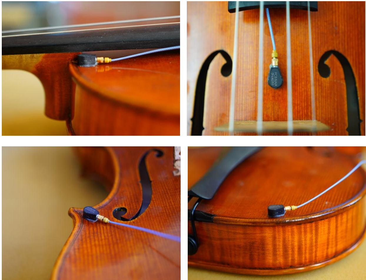
FIGURE 5.11. Accelerometer placed at various locations on the expensive violin: point 1 (top left), point 31 (top right), point 40 (bottom left), and point 67 (bottom right).
