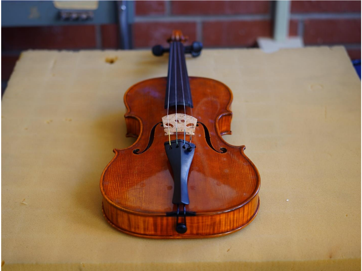
FIGURE 5.9. A foam pad was used to mitigate stray vibrations during vibrations and acoustic testing.
