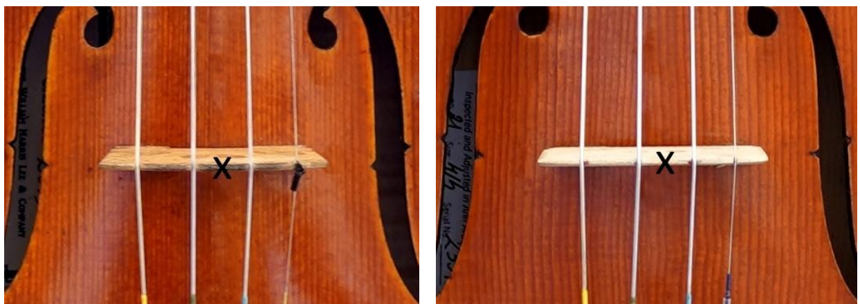
FIGURE 5.17. Bridge excitation location on expensive violin (left) and cheap violin (right). The excitation point is on the central top of the bridge.
