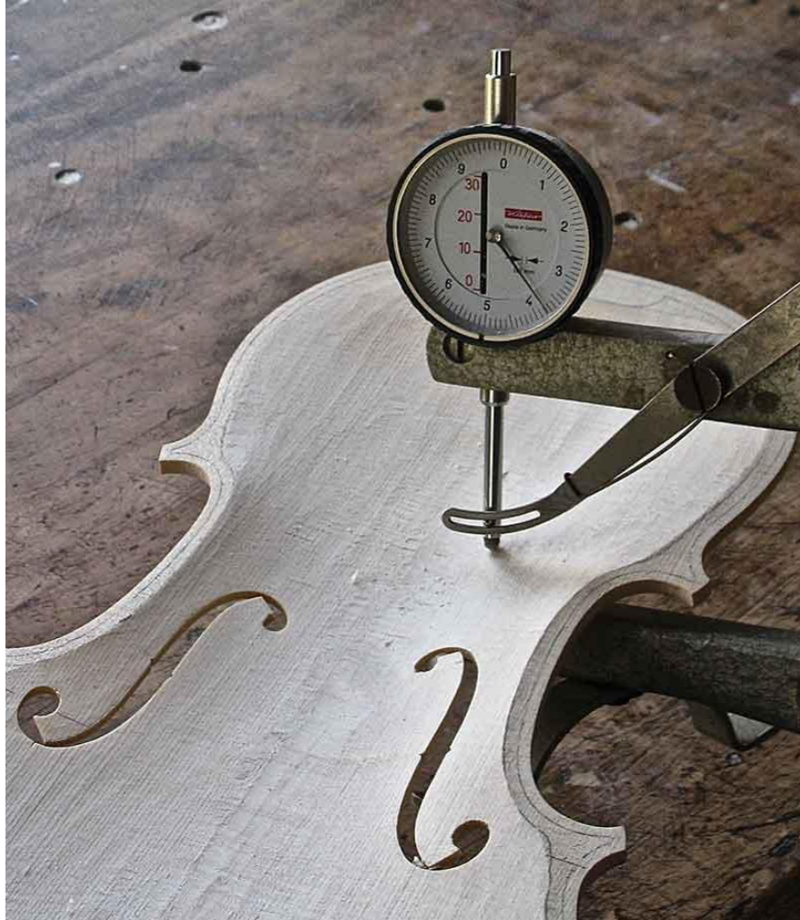
FIGURE 1.10. Graduating caliper used to check the thickness of a violin top plate [20].
