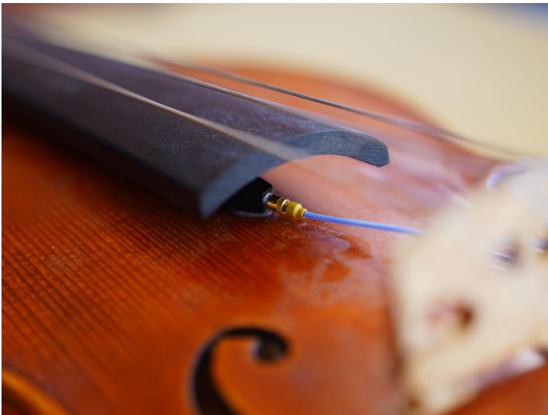
FIGURE 5.12. Placement of an accelerometer at point 21, under the fingerboard. The small size of the accelerometer allows for placement in cramped areas.
