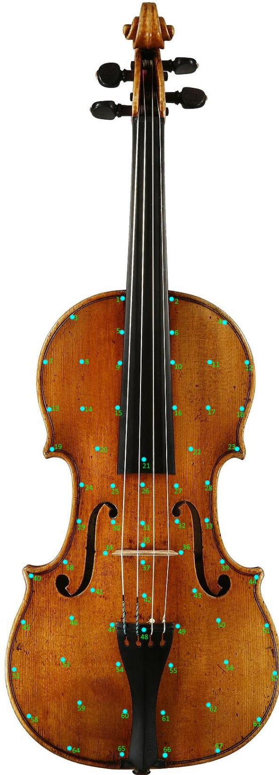
FIGURE 5.10. 67 accelerometer test points.
